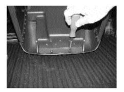
**STEP 11: (a)**With lid removed, remove the T-15 Torx screws.
