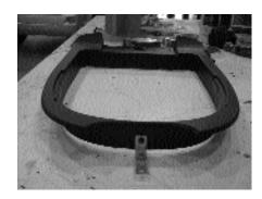
**STEP 17: (c)** Mount the small angle bracket using the supplied black rivet and small washer.
