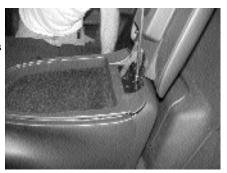
**STEP 21:** Mount the OEM strap using the "7th" T-15 Torx bolt
