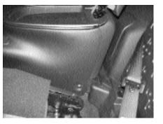
**STEP 14:** From inside of the truck, place the outer OEM shell over the Stealthbox®®.
