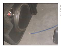
**STEP 4**Run speaker wire from the amplifier's location to the Stealthbox' location and check for proper operation of
