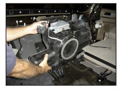
**STEP 22**Remove the woofer system from the SUV.
