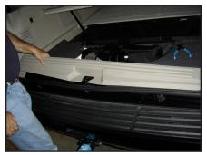
Remove the tailgate's lower sill plate.
