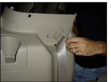
**S T E P 1 8**Pull the front portion of the side panel from location. Feed the second row seat belt through the opening of the side panel.
