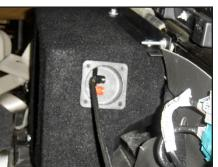
Run speaker wire from the amplifier location to the Stealthbox® location.
