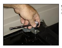
**S T E P 1 6**With an 8mm socket, remove the bolt that secures the side panel metal bracket to the floor.
