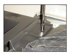
**S T E P 4**With an 8mm socket, remove the bolts that secure the plastic storage bins to the floor.
