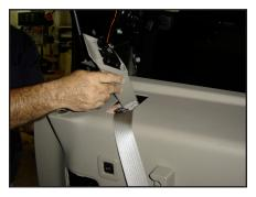
**STEP 17**Pull the rear portion of the side panel from location. Feed the third row seat belt through the opening of the side panel.
