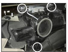
**S T E P 2 1**With 10mm socket, remove the two nuts and one bolt that secure the plastic woofer enclosure to the SUV.
