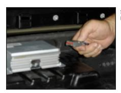
**STEP 20**Remove the plug from the factory amplifier.
