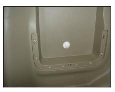
**S T E P 4**Drill a 1" hole in the interior panel where marked as **STEP 3** as shown.
