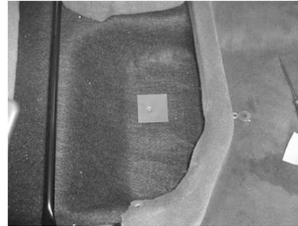
**STEP 5:** The threaded rod will leave an impression, onto the wax square.
