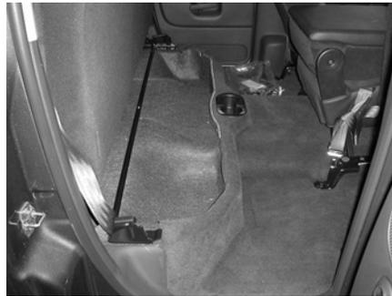
**STEP 1:** Remove the passenger side metal floor extension, if so equipped.
