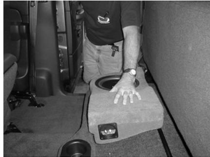
**STEP 4:** Place the Stealthbox into the passenger's side cavity and push down.
