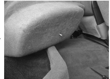
**STEP 3:** Thread the supplied socket set screw into the Stealthbox. Leaving 1/2" exposed.
