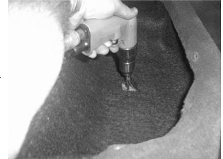
**STEP 6:** With a 1/2" drill bit. Drill a hole into the floor using the imprint in the wax square as guide.
