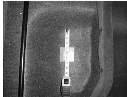
**STEP 2:** Remove the paper backing and place supplied wax square onto the floor:
