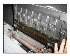
**STEP 4**Remove the driver's and passenger's side folding floor extensions.
