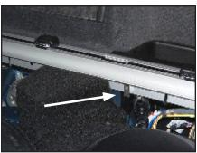
**STEP 12**Slide a U-Nut over the factory hole in the rail, as shown.
