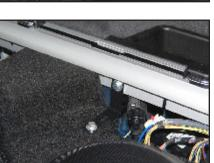
**S T E P 1 3**Secure the Top Bracket to the Stealthbox® and to the rail using a pair of 1/4" - 20 x 1" Bolts, 1/4" Lock Washers, and 1/4" Flat Washers.
