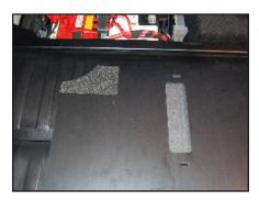
**S T E P 1 4**Cut the Foam Tape into three 4" strips, affix them to the new Battery Cover, and trim away the excess, as shown.
