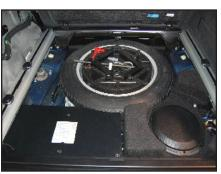
Secure the Battery Cover using the three #8 x 1" Screws.
