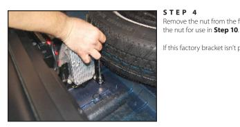
**S T E P 4**Remove the nut from the factory bracket, as shown. Retain
