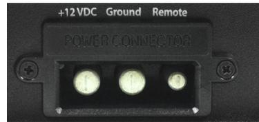
You can identify the older HD750/1 and MHD750/1 by the plastic trim around the area the plug connects to the amplifier. In the image above, note the screws on either side of the opening.
