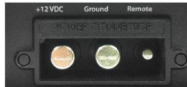
You can identify the newer HD750/1 and MHD750/1 by the plastic trim around the area the plug connects to the amplifier. In the image above, note the larger overall size and the LACK of screws on either side of the opening.
