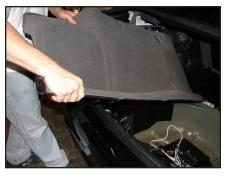
**STEP 3** Remove the driver's side trunk liner as shown.
