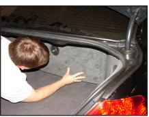
**STEP 13** Slide the Stealthbox<sup>®</sup> into position with the drivers side going in first (see **STEP 14**).
