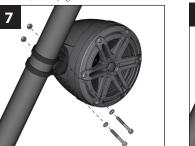
Realign the clamps with the clamp receiver on the enclosure, and secure them to the clamp receiver using a pair of Mo x 45 mm Machine Screws, M6 Flat Washers, and M6 Locknuts as illustrated, and fully tighten. Note: The locknut should be installed into the hex shaped
