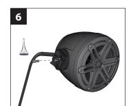
Remove the center M6 x 16 mm Machine Screw from the clamp receiver, apply Loctite\* red thread-locking compound, reinstall, and fully tighten.
