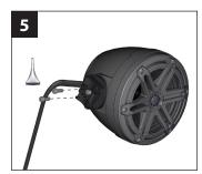
Apply Loctite\* red thread-locking compound to two M6 x 16 mm Machine Screws, slide them through the slots in the clamp receiver, into the appropriate holes in the fixture base, and fully tighten.
