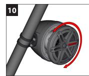
Rotate the speaker to the desired angle. Reinstall the speaker and speaker mounting screws and washers. Hand-tighten in a criss-cross pattern.
