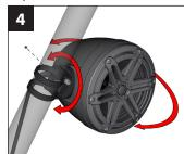
Position the enclosure at the desired location, tightening the M6 x 45 mm Machine Screws as necessary. Fully tighten the pre-installed M4 x 4 mm Set Screw in the clamp receiver to hold its position. Mark the location of the clamps on the pine: then remove the enclosure
