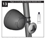
Clean the inside of the aluminum cap with acetone (not included) prior to attaching it to the enclosure. Apply a circular bead of silicone adhesive to the inside of the aluminum logo cap, 1/2-inch (13 mm) from the outer edge.
