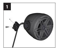
Loosen the pre-installed M4 x 4 mm Set Screw in the clamp receiver. Slide an M6 x 16 mm Machine Screw through the center hole of the clamp receiver, into the center hole in the fixture base, and hand tighten.
