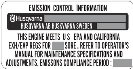
The Emissions Compliance Period referred to on the Emission Compliance label indicates the number of operating hours for which the engine has been shown to meet Federal and California emissions requirements.
