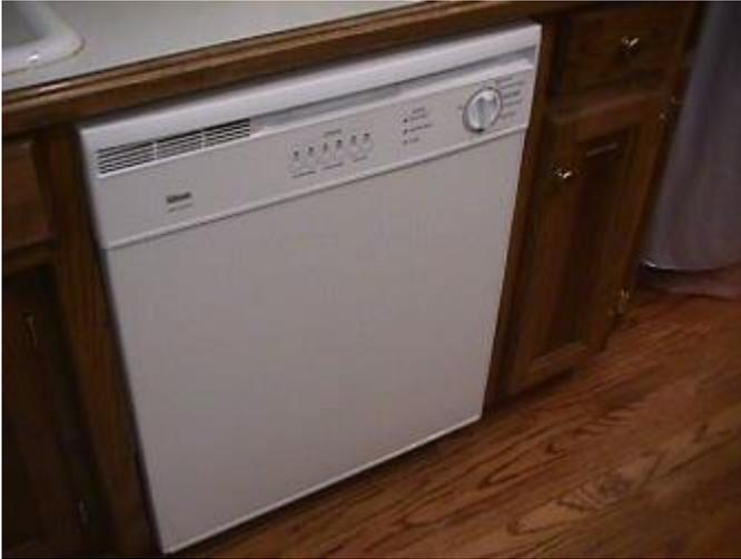
Cabinet mount dishwashers have two screws under the counter lip, holding them in place. Remove these two screws and slightly bend downward the attaching brackets. This will prevent the bracket from catching the bottom of the counter surface and scratching the surface.
