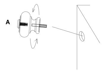
The Bun Feet (A) are packed in a individual box, and placed in case or bottom of case.
