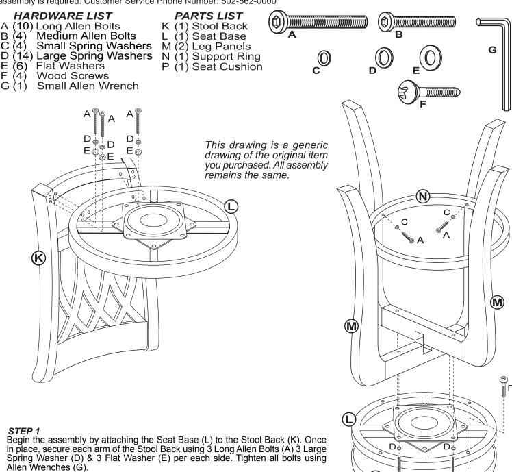
Attach each Leg Panel (M) together by sliding each into place. During assembly, secure the Support Ring (N) to the inside of each leg using 1Long Allen Bolts (A) & 1 Spring Washer (C) per each leg. Tighten all bolts.
