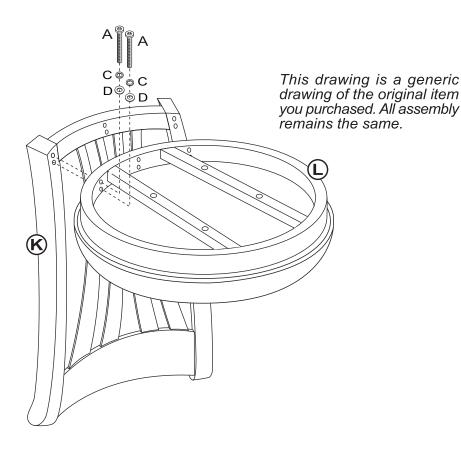
**STEP 1** Begin the assembly by attaching the Seat Base (L) to the Stool Back (K). Once in place, secure each arm of the Stool Back using 2 Long Allen Bolts (A) 2 Spring Washers (C) & 2 Flat Washers (D) per each side. Tighten all bolts using Allen Wrenches (É).
