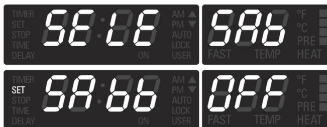
3. Touch **MENU** to enter edit mode: SAbb is shown on the left and its status is shown in the right field, blinking.
