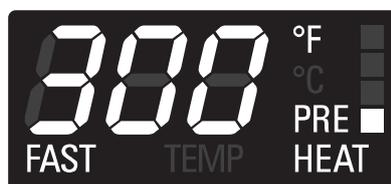
As soon as the set-point temperature is reached, the control sounds an "end of preheat" tone and both "FAST" and "PREHEAT" disappear. The oven switches to the cooking mode set: put the food inside now.
