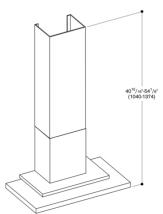
\* Suitable for ceiling heights of 8.7 ft (2.64 m) to 9.7 ft (2.97 m); Specifications refer to a distance from floor to lower chimney edge of 5.2 ft (1.60 m).
