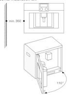
When using the  $92^{\circ}$  door hinge restrictor (Spare Part No. 00636455), the minimum distance to the wall is only 100 mm.
