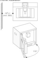
If using the 92° door hinge restrictor (spare part no. 00636455), the minimum distance to the wall is only  $3^{15}/1e^{\alpha}$  (100 mm).
