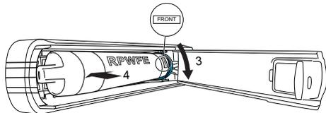
4. While continuing to ensure cartridge is fully seated in the holder, gently swing the filter inward until it is in position. If filter will not swing easily, check to ensure filter is properly aligned and fully seated within the cartridge holder.
