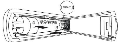
4. While continuing to ensure cartridge is fully seated in the holder, gently swing the filter inward until it is in position. If filter will not swing easily, check to ensure filter is properly aligned and fully seated within the cartridge holder.
