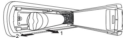
2. When the cartridge can no longer swing, gently pull to unseat it from the cartridge holder. A small amount of water may drip out.
