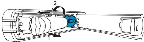
2. Twist the cartridge one-quarter turn **counter-clockwise**. After twisting, remove the cartridge by pulling it away from the cartridge holder. A small amount of water may drip out.
