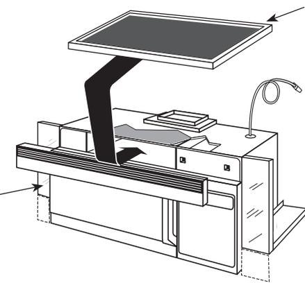
Filter Kit JX81L-Recirculating Charcoal Filter Kit To be used when the Spacemaker microwave oven cannot be vented to the outside.
