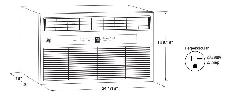
Note: When installing units in through-the-wall applications.
