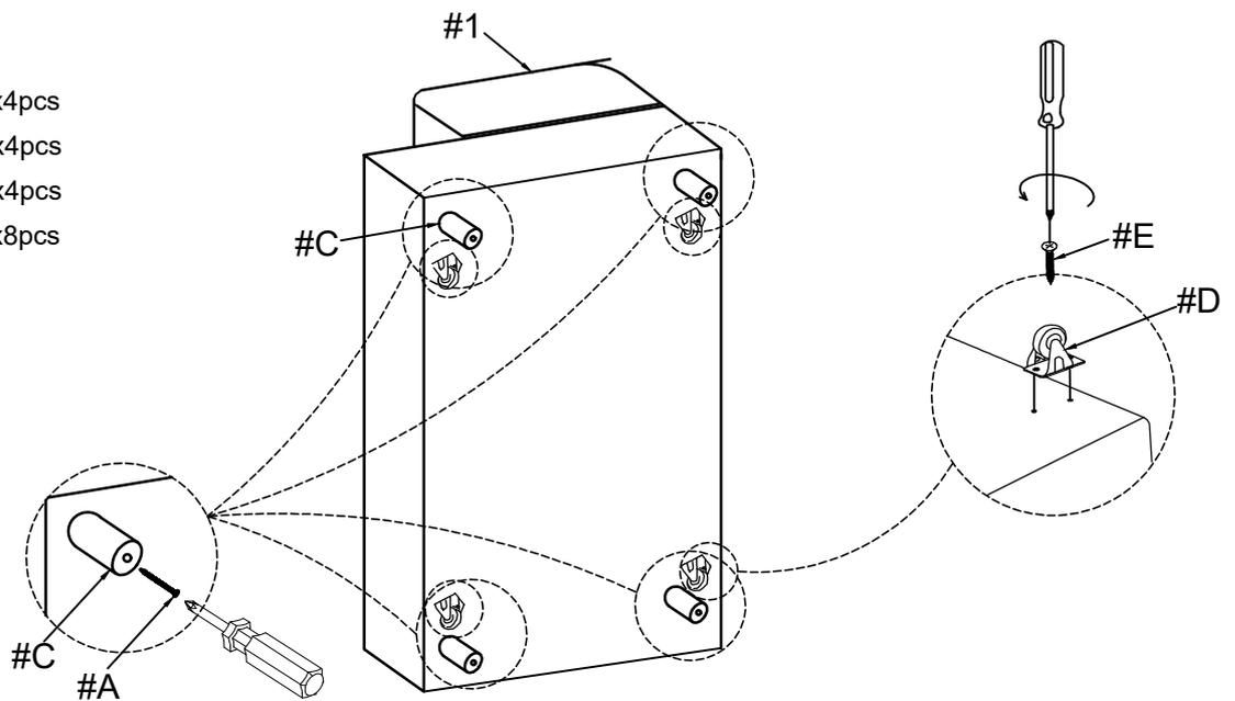
Align legs (#C) and wheels (#D) to the bottom of loveseat (#1), then secure by using screws (#E). There will be no pre-drilled holes on the bottom of the loveseat (#1).
