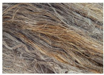
Flax offers unique qualities: light because it is hollow and very low elasticity. It constitutes a choice suitable for the manufacture of the core of a sandwich structure.
