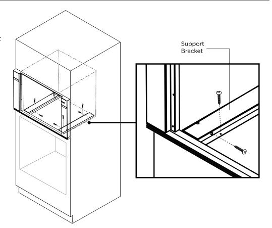
Fit the 4 supplied rubber plugs into the Trim Surround in the correct hole positions, as shown.
