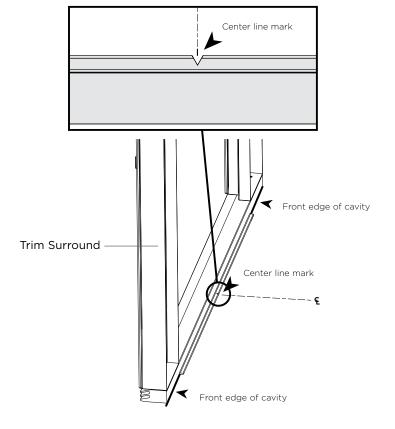
Using the 4 supplied screws, secure the Trim Surround to the cabinetry in the correct hole positions, as shown.
