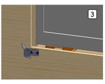
of the magnet mount as required to fine-tune the alignment between the EuroTrim™ and the microwave. Next, open the microwave door and check for proper clearances. Adjust the alignment of the EuroTrim™ by removing it briefly and repositioning the flaps of the magnet mount until you are satisfied. (3)
