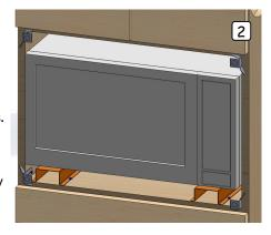
Adjust until you are satisfied with the placement. Next, remove the EuroTrim<sup>™</sup> without moving the microwave. (2)
