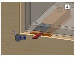
the microwave. After initial contact firmly press them onto the runners. <u>Hint</u>: Lift the microwave up at the front and push it back far enough to rest the feet temporarily on the STOPADS©. Next, wiggle the handle of the STOPADS© horizontally until they break off. Then, pull the microwave toward you until the feet come to a rest inside the STOPADS©. (4)
