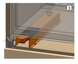
Next, wiggle the handles of the STOPADS© horizontally until they break off. Then, pull the microwave toward you until the feet come to a rest inside the STOPADS©. (3)
