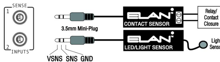
Available ELAN sensors include: AUDIO, VIDEO, CONTACT CLOSURE, VOLTAGE, LED/LIGHT, and CURRENT/MAGNETIC FIELD sensors.
