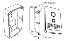
Place the video doorbell on the mounting hooks and slide the video doorbell down.
