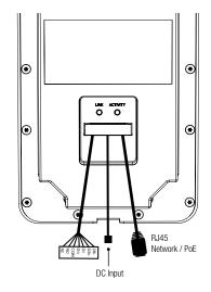
Note: the RJ45 connector block should be on the right side of the terminal connector, as shown here.
