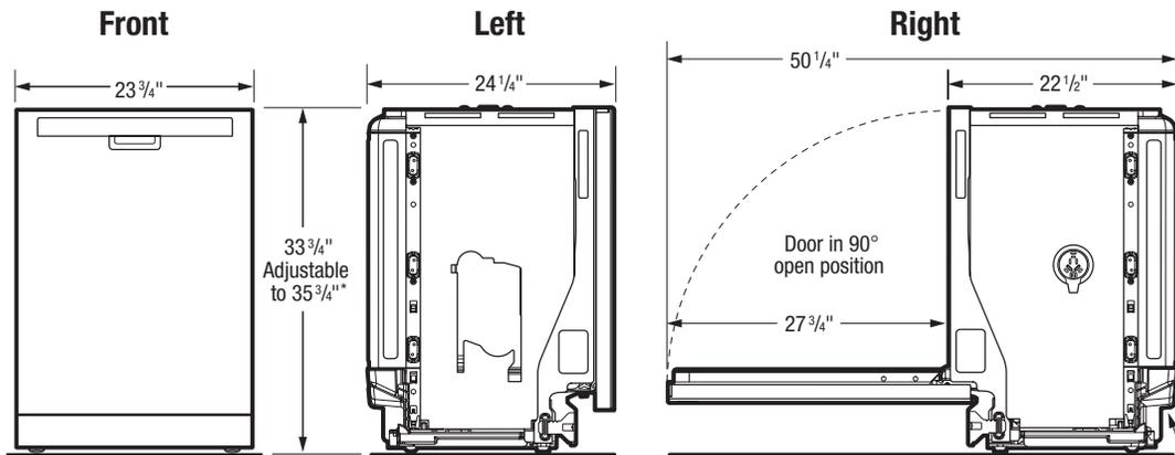
\*Height only adjustable to 35 3/4" max. when installed in 35 3/4" max. standard cabinetry cutout. (Dimensions do NOT include insulation – insulation blanket may be compressed during installation.)
