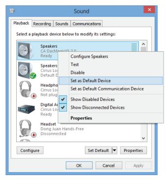
7. Go to the Speakers Properties of the DacMagic XS and choose the sample rate output.
