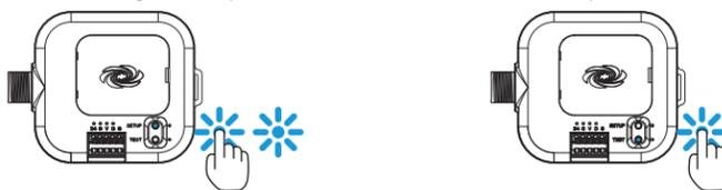
Pressing any button on a device that is part of the network takes the system out of joining mode. Joining mode ends automatically after 4 minutes.
