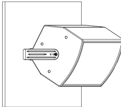
**WARNING:** Loudspeakers cannot be vertically mounted on a wall as shown in the following diagram.
