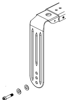
4. Tighten the socket head cap screw to secure the loudspeaker in the bracket.
