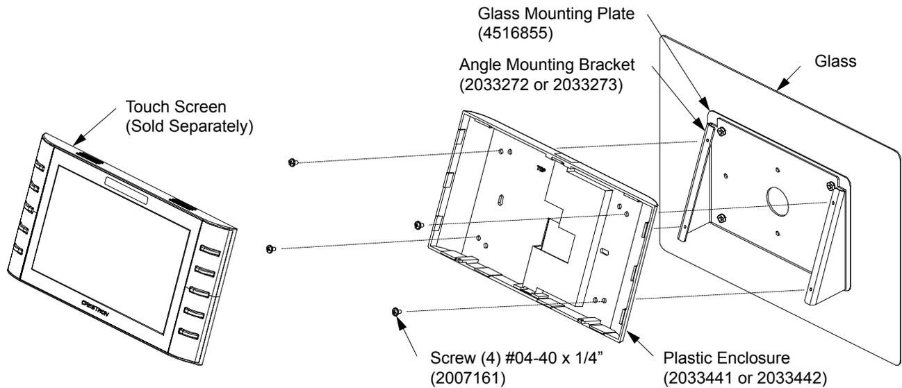
5. Secure the touch screen to the plastic enclosure with Phillip head screws. Alternatively, security Torx screws can be installed using a Torx screwdriver bit (both included with touch screen), as shown in the illustration on page 8.
