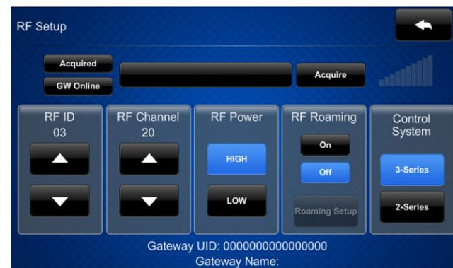
3. When the screen displays an "Acquire OK" message, press **ACQUIRE** on the gateway to exit Acquire mode. The LED turns off.
