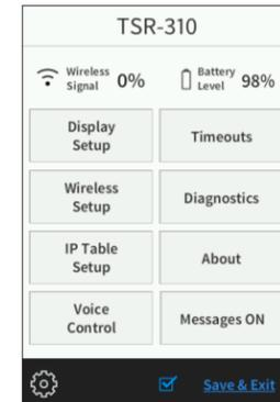
To access the setup screens during normal operation, press the power (1), microphone (2), home (3), and raise volume (4) buttons twice, in this order, within five seconds. Refer to the illustration below for button locations on the TSR-310.
