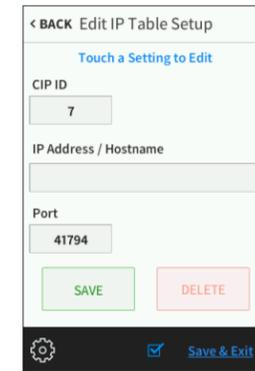
3. Tap the text field below **CIP ID** to enter the appropriate CIP ID using the on-screen keypad.
