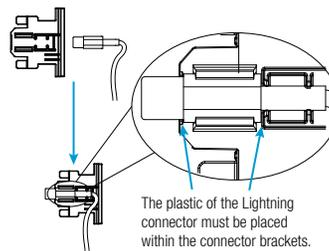
6. Place the cable holder containing the Lightning to USB cable in the iPad.
