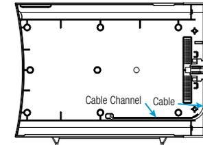
8. Replace the metal plate and secure it to the iPad using the screws and washers removed in step 3.
