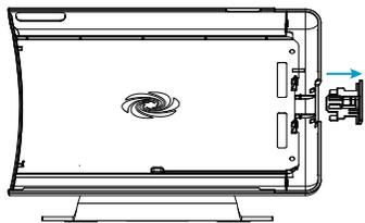
3. Use the Phillips screwdriver to remove the screws and washers that hold the metal plate in place, and remove the metal plate.
