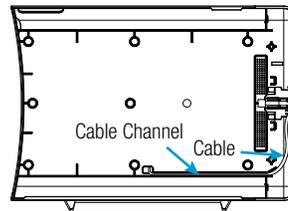
5. Snap the Lightning connector of the Lightning to USB cable in the cable holder.
