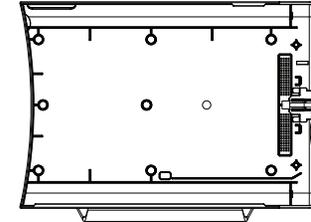
7. Starting from the connector, loosely place the cable in the cable channel and press it into the channel to secure it.
