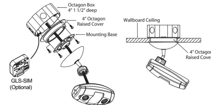
**Option C. Surface Mount Raceway Installation**
