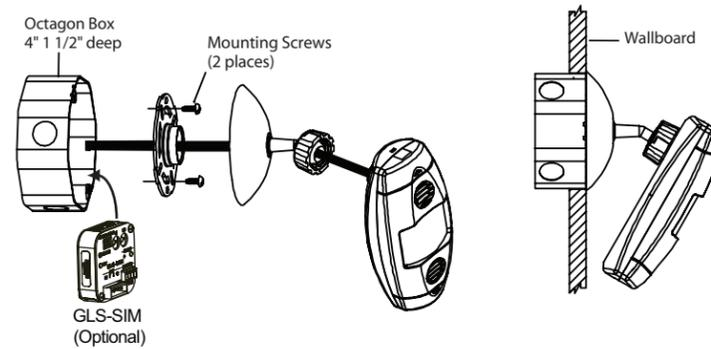
**Mounting to Octagon Back Box Installed Flush to Drop Ceiling**
