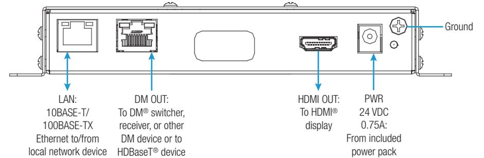
**NOTE:** The DM OUT port is a PoDM (Power over DM) and HDBaseT® PoE (Power over Ethernet) PD (Powered Device) port. To receive PoDM or HDBaseT PoE, the DM-TX-201-C requires a connection to a DM® switcher or other equipment that has a PoDM or HDBaseT PoE PSE (Power Sourcing Equipment) port. Any wiring that is connected to a PoDM or HDBaseT PoE PSE port is for intrabuilding use only and should not be connected to a line that runs outside of the building in which the PSE is located.
