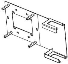
2. Using the four included 6-32 x 3/4" combo truss head screws, attach the included support bracket to the electrical box.
