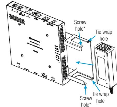
\*Use either screw hole for the included 6-32 x 1/2" Phillips pan head screw.
