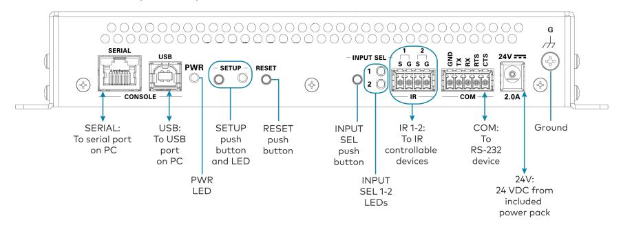
Rear Panel Connections - DM-NVX-350 and DM-NVX-351
