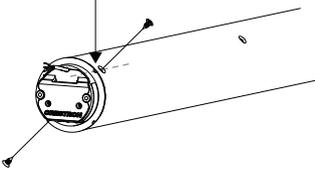
3. Rotate the motor head so that the groove in the motor is shown through the second screw hole in the roller tube.
