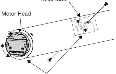
Rotate the motor head until the groove is visible through the screw hole, and then install the screws.
