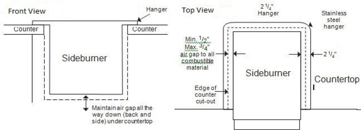
The two top illustrations demonstrate how the slide-in type unit is designed to fit into open- front enclosures, and supported at the Countertop.
