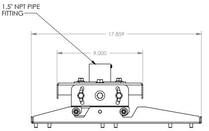
X = TOP OF 1.5" NPT FITTINGDOWN TO CENTER OF LENS.
