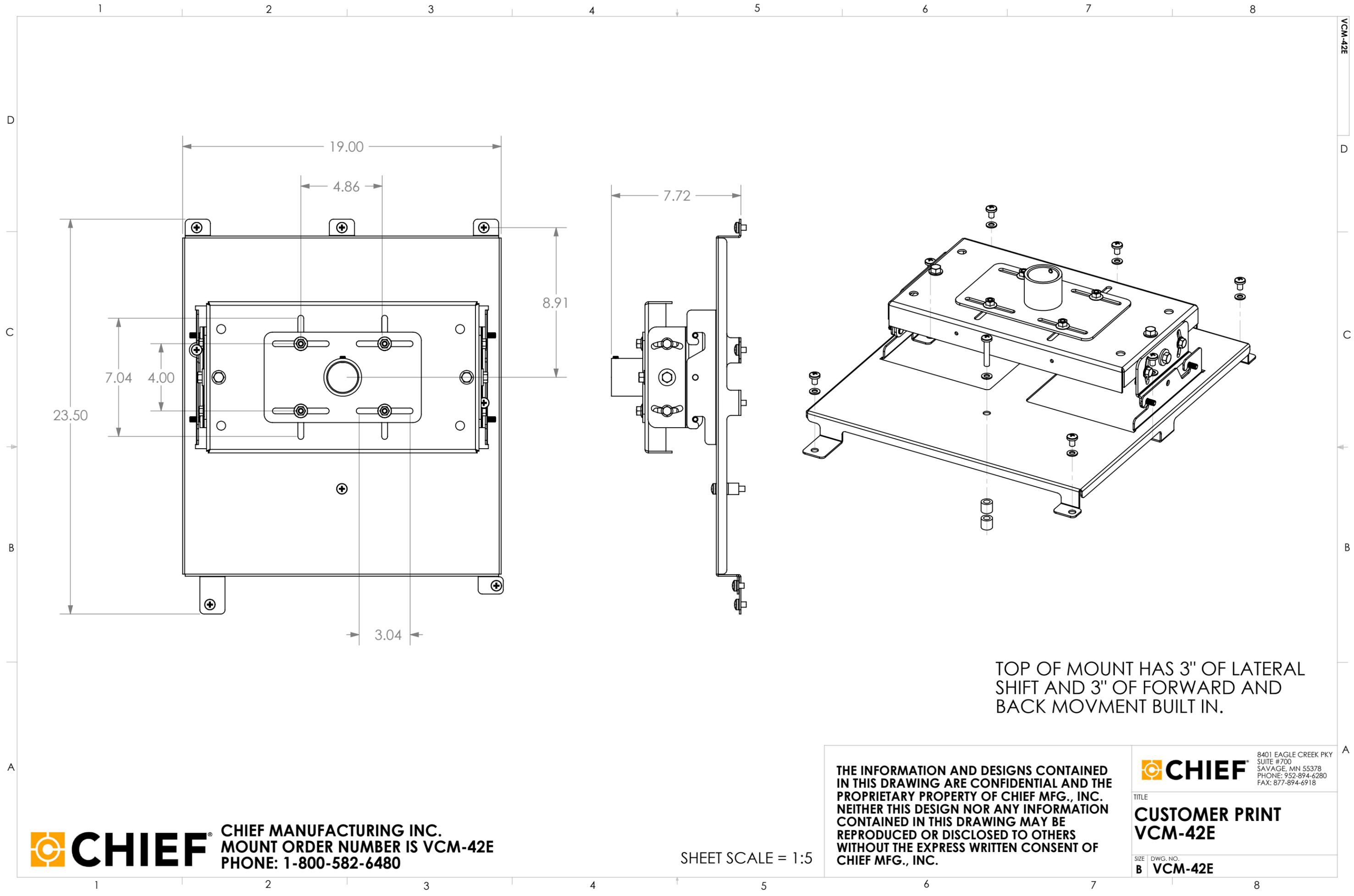
TOP OF MOUNT HAS 3" OF LATERAL SHIFT AND 3" OF FORWARD AND BACK MOVMENT BUILT IN.
