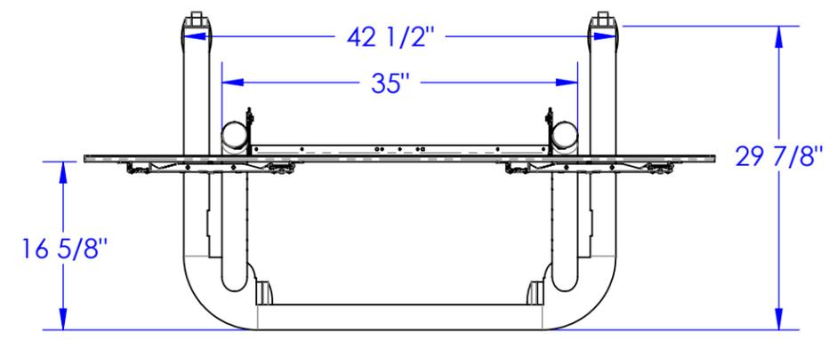
NOTE: CUSTOM INTERFACE BRACKET NOT SHOWN. THE CUSTOM INTERFACE BRACKET NEEDED FOR YOUR DISPLAY WILL ADD BETWEEN 1/2" AND 2" IN DEPTH AND MAY AFFECT LOCATION OF DISPLAY ON THE MOUNT.
