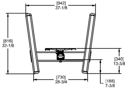
NOTE: CUSTOM INTERFACE BRACKET NOT SHOWN. THE CUSTOM INTERFACE BRACKET NEEDED FOR DISPLAY WILL ADD BETWEEN 1/2" AND 2" IN DEPTH AND MAY AFFECT LOCATION OF DISPLAY ON THE MOUNT.
