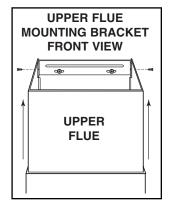
Screw from top of hood base. Do not overtighten these screws.
