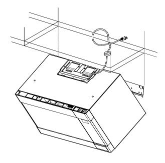
This model can also be installed for external venting. For full installation details and requirements consult the installation manual.
