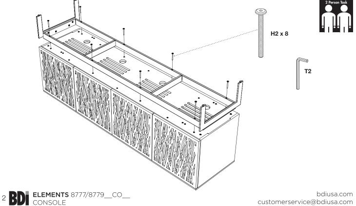
**Step 3 Triple -** With help from another person, carefully position the cabinet **A1** upside-down (as shown) or on its back. Attach the base to the cabinet with **8 Screws H2** using **Hex Wrench T2.** Do **NOT** fully tighten until all 8 screws are started.
