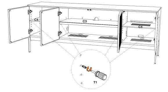
**Step 6 -** The 2 **Back Panels C5** are removable and can slide towards the middle. To remove lift up and pull the bottom edge out of its groove. To re-install, put the top edge of the back panel into the top groove, then drop the bottom edge into the bottom groove.
