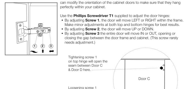
on this hinge will close the seam between Door C & Door D here.....
