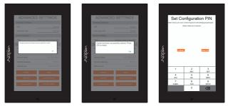
Device Settings - The touch pad can be renamed for easier syncing with Velocity. Type the name into the **Alias** field.
