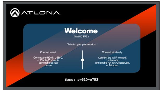
The splash screen will show the OSD (On-Screen Display). The splash screen will display instructions on connecting devices wirelessly or by connecting directly to the AT-UHD-SW-510W, using cables. The SSID or the AT-UHD-SW-510W will be displayed at the bottom of the screen.
